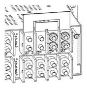
(The image above shows typical 2U panel application—wire ready. Trimm part number 7510131540)
